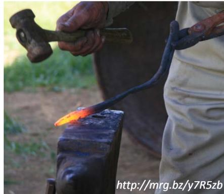
*Blacksmith hot forging a steel tool using a hammer and an anvil.*
