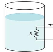
**Figure 1:** Electric resistance heater in a tank of water.
