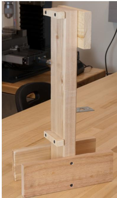
Figure 2: Photograph of an assembled fish tank platform before it is painted.
