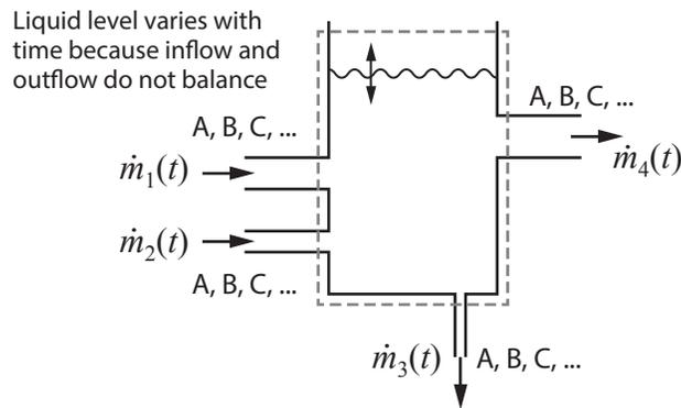
**Figure 3:** Unsteady flow model of a mixing process.
