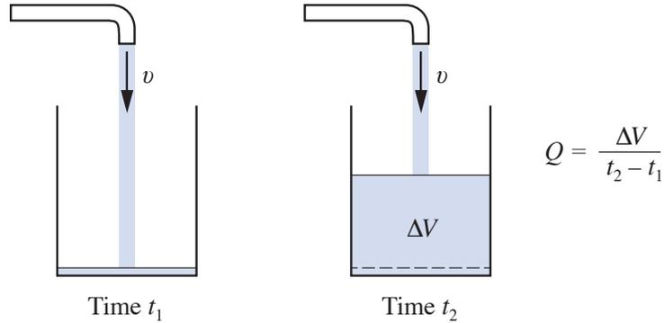
**Figure 4:** Volumetric flow rate during the filling of a bucket. The flow rate is assumed to be steady.
