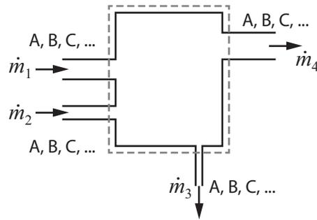
**Figure 2:** Steady flow model of a mixing process.
